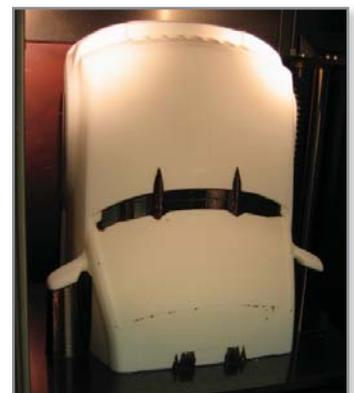
Figure 6: 1/4 scale part built on FDM Maxum
