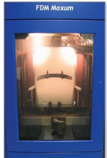
Figure 11: Scale model is built on an FDM Maxum
