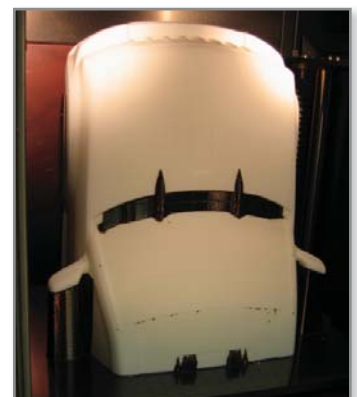
Figure 6: 1/4 scale part built on FDM Maxum
